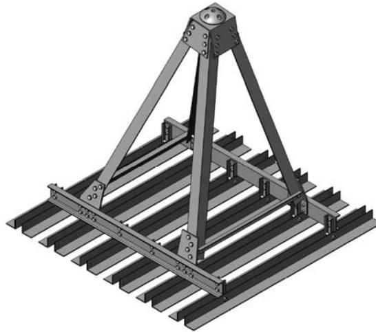
**Figure 4: Three dimensional CAD model of mast foundation**
